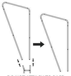
DO NOT ATTACH TO BASE UNTIL GRAPHIC IS INSTALLED
